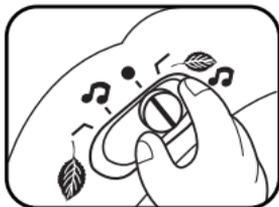
2. Locate the battery cover on the back of the unit. Use a coin or screwdriver to loosen the screw.
