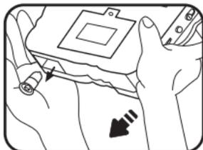
4. Attach the protection ring to the new light bulb. Place the protection ring around the new light bulb and turn the ring until it is securely fastened to the new light bulb. Carefully put the new light bulb into the light bulb socket. Please use a 4.8 volt, 0.3 A light bulb. Please note the maximum power light bulb that can be used is a 2.4 watt light bulb.
