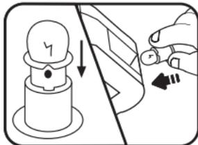
5. Replace the light bulb cover and secure the screw using a coin or screwdriver.
