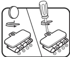
4. Replace the battery cover and tighten the screw to secure the battery cover.
