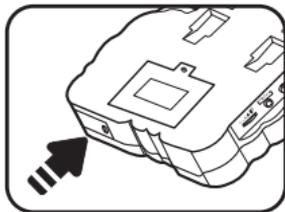
2. Make sure the unit is turned **OFF**. Use a coin or screwdriver to open the cover.
