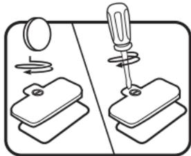
3. Install 4 new "C" size (UM-2/LR14) batteries following the diagram inside the battery box. (The use of new alkaline batteries is recommended for maximum performance.)
