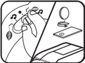
3. Gently pull out the old light bulb and remove the protection ring from the old light bulb.
